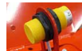
Fill Level Sensor Signals when hopper is low on seed.
