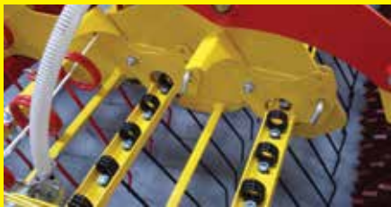
Adjustable 8mm tines allow for more or less aggressive field operation.
