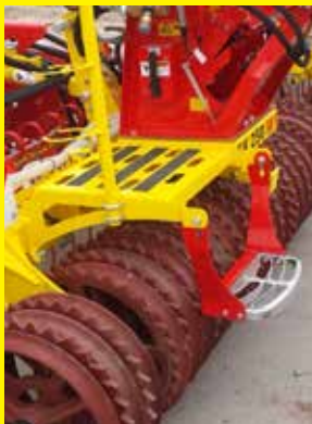
Seeder access platform
