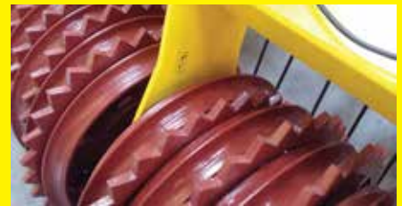
Cambridge roller for existing grass operations.
