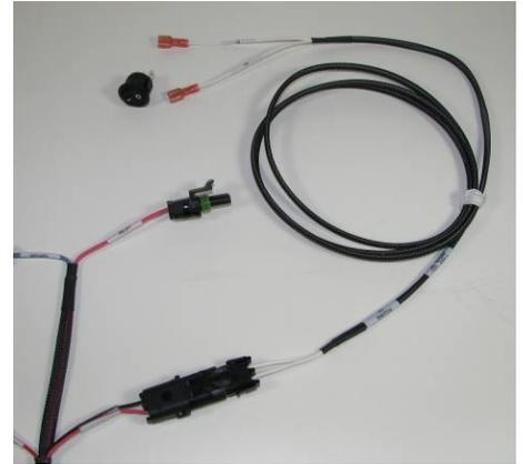
3. Connect the cable labeled R7 Switch to the switch pins.
